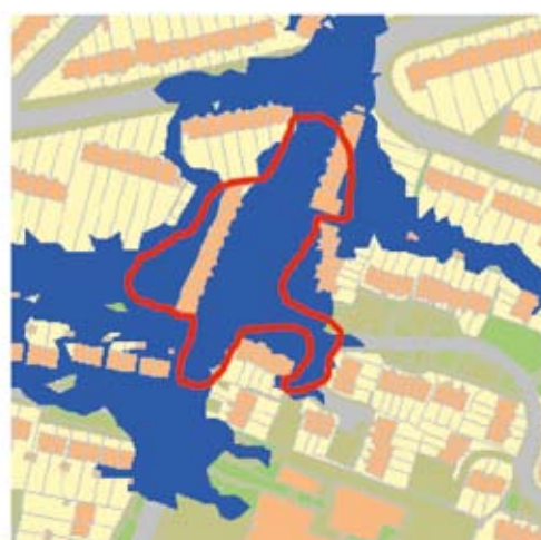
b) Decoupled sewer model and 2D overland routing
